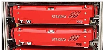
The new Stingray shuttles that will serve the automated forward stock picking system have been delivered. We have purchased a total of 115 shuttles that will move between 90,000 different stock locations.
