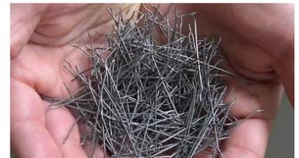
As detailed above, we are mixing steel fibres with concrete to reinforce the floor. Across more than 200,000 square metres of flooring, our building contractors estimate that we will use a staggering total of 201 billion fibres!
