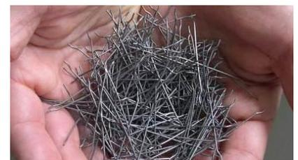
As detailed above, we are mixing steel fibres with concrete to reinforce the floor. Across more than 200,000 square metres of flooring, our building contractors estimate that we will use a staggering total of 201 billion fibres!
